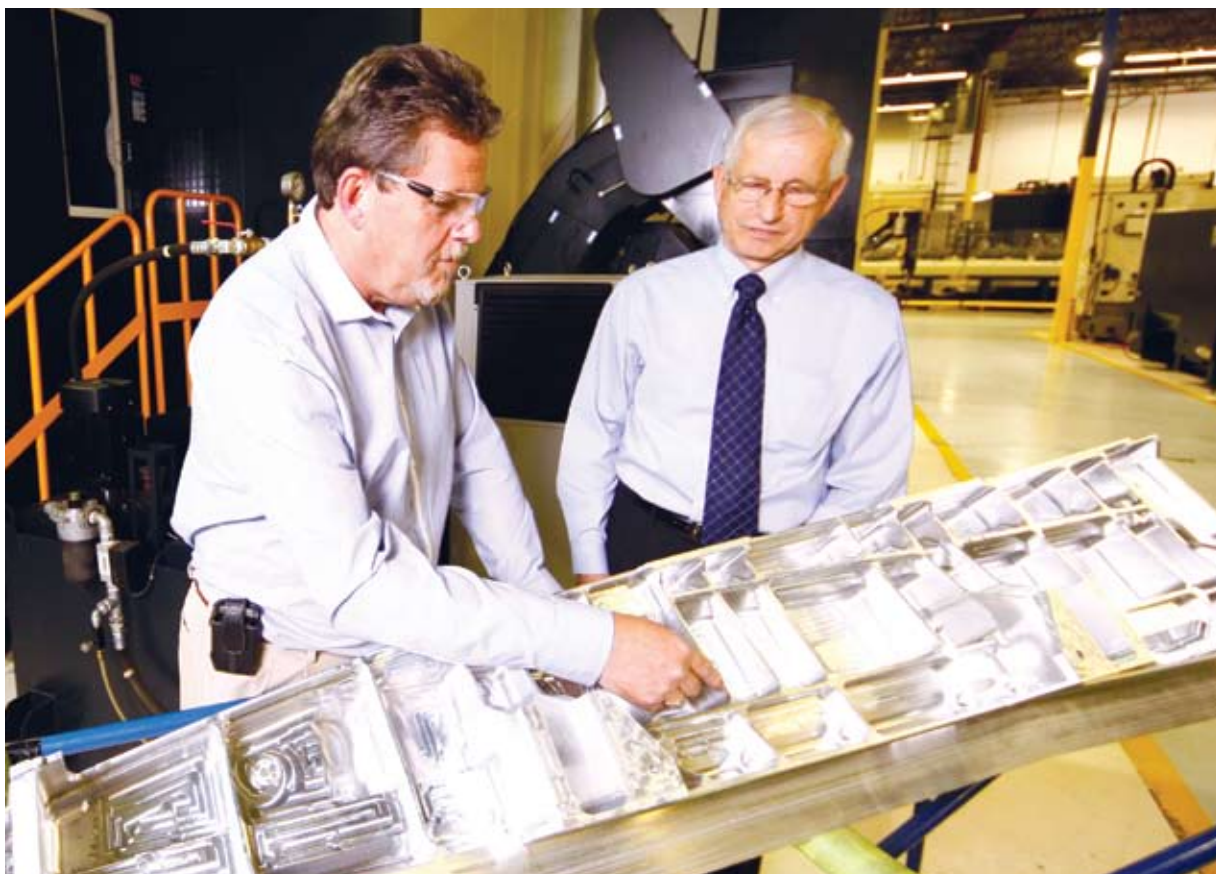
Vic Gerden (right), Executive Director of the Manitoba Aerospace Association, and Vince Martin, President, Cormer Aerospace, discuss the capabilities of the MAG 3 high-speed 5-axis machine at Cormer which is the latest technology in precision machining. This machine is one of few in Canada and runs 'lights-out' with its large 10-place automatic pallet system. They are examining one of the 787 monolithic engine parts that this machine produces.
