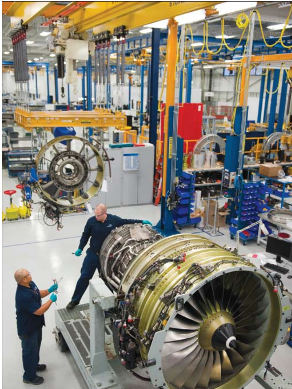
Technicians at StandardAero work on a CFM56 engine at the company's repair and overhaul shop in Winnipeg. The CFM56 engine powers the 737 and other single-aisle airline planes, which account for a large bulk of passenger aircraft worldwide.
